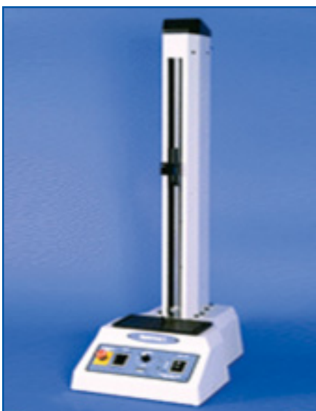
Tensile strength testing machine
